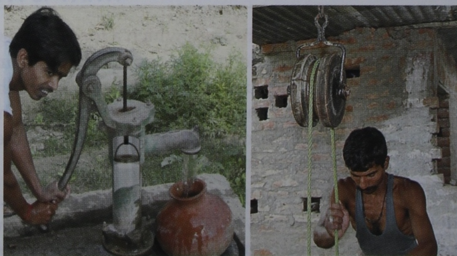
Fig. 5.3 The handle of a hand pump and a pulley change the direction in which force is applied.
