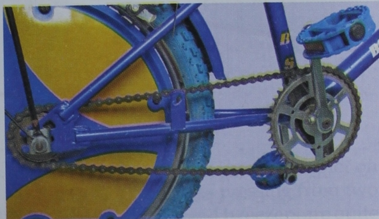
Fig. 5.5 The cogwheel of a bicycle helps you gain speed.
