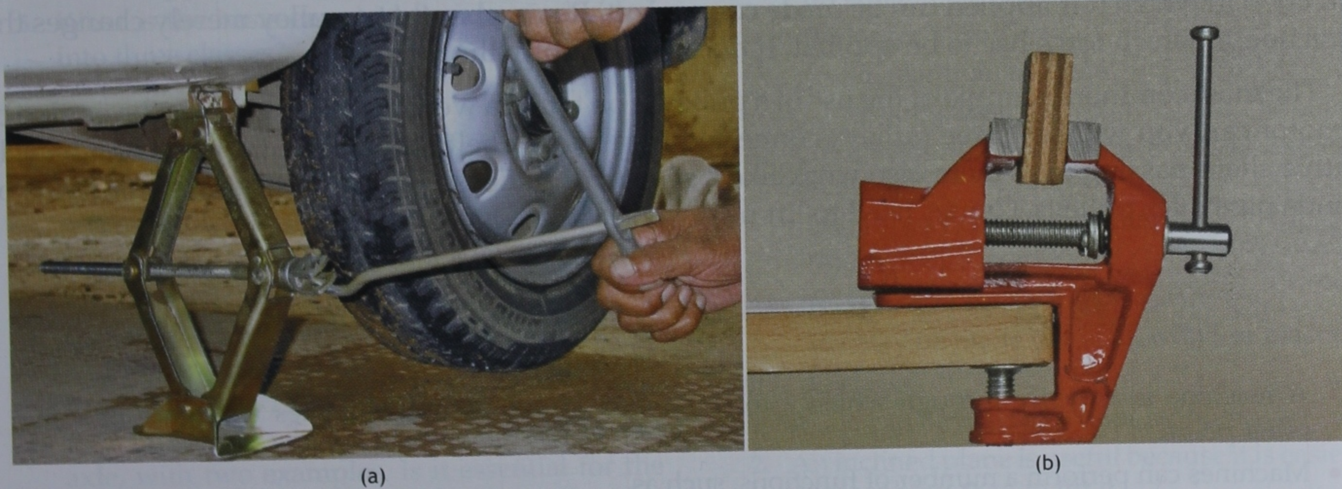
Fig. 5.14 (a) A car jack and (b) a vice are applications of the screw.
